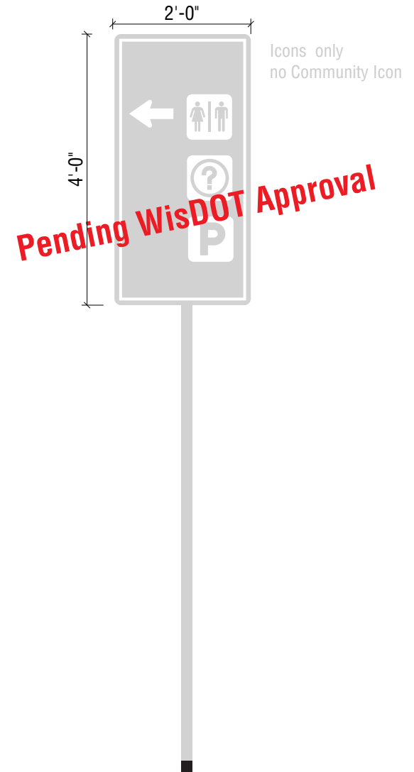
3.1c New Structure 2" Steel posts painted Black
