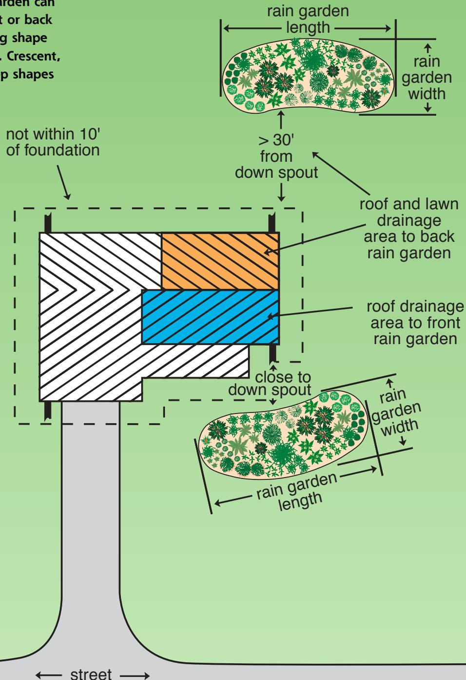
**Figure 2** Rain gardens should be located at least 10 feet from the house, on a gentle slope that catches downspout water.
